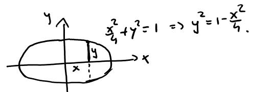
$$\begin{aligned} \therefore V &= 2 \int_0^2 \frac{1}{2} \pi (1 - \frac{x^2}{4}) dx \\ &= \pi \left( x - \frac{1}{12} x^3 \right) \Big|_0^2 \\ &= \pi \left( 2 - \frac{1}{12} 8 \right) = \boxed{\frac{4}{3} \pi} \quad (\text{cubic units}) \end{aligned}$$
