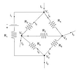
The jagged lines correspond to resistors. The pair of parallel lines corresponds to a voltage source of e volts. Let  $I_0, I_1, I_2, I_3$  denote the input currents at each of the corresponding nodes, let  $i_1, i_2, i_3, i_4, i_5, i_6$  be the currents through the various branches, as indicated, let  $V_0, V_1, V_2, V_3$  be the voltages at each node and let  $R_1, R_2, R_3, R_4, R_5, R_6$  be the resistance at each of the resistors in the diagram. Assume that  $V_0 = 0$ . Finally, we set
